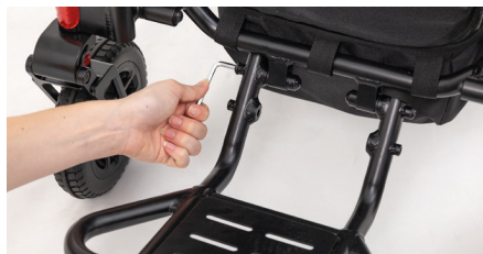
Figure 1: Desserrez les vis
